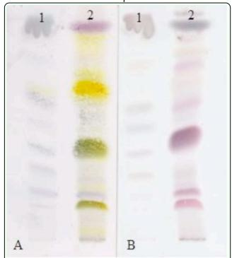
**Figure 1.** Thin layer chromatography of seed (1) and fruit (2) extracts of *Cabralea canjerana* obtained with ethyl acetate developed with vanillin sulfuric acid (A) and copper sulfate (B). High quality figures are available online.
