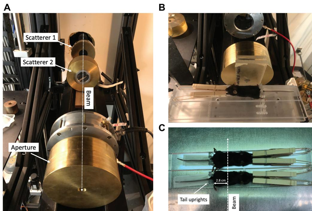
**FIG 1.** The experimental set-up enables irradiation of two mice at the same time. Mouse phantoms and Monte Carlo simulations are used to evaluate the dose. Panel A: The double-scattered system. Panels B and C: Mouse holders used for the reproducible immobilization. The beam can go through two parallel mice laterally.
