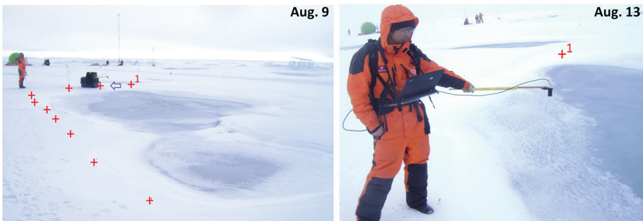
FIGURE 5. Repeated measurements of albedo transects (top) passing through the same melt pond (bottom). The interval between red crosses is 100 cm. the first location on snow is marked in both photos, with last two locations also on snow (MP S/I means a mixture of melt pond snow and ice; water means melt pond water).
