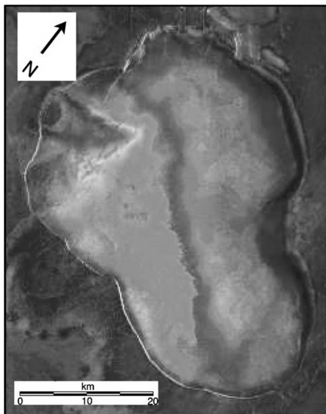
FIGURE 5. SAR interferogram of the Vavilov Ice Cap, derived from a pair of SAR images acquired on 15 and 16 May 1996, during the ERS Tandem Phase. The interferometric baseline between the two satellite locations is 1 m. The interferogram is still in SAR slant-range coordinates, with a view direction from left to right. Each fringe (i.e., one complete cycle through the color scale) represents a velocity change of 10 \text{ m a}^{-1} in the look direction of the ERS satellite. The interferogram was processed by A. Shepherd.
