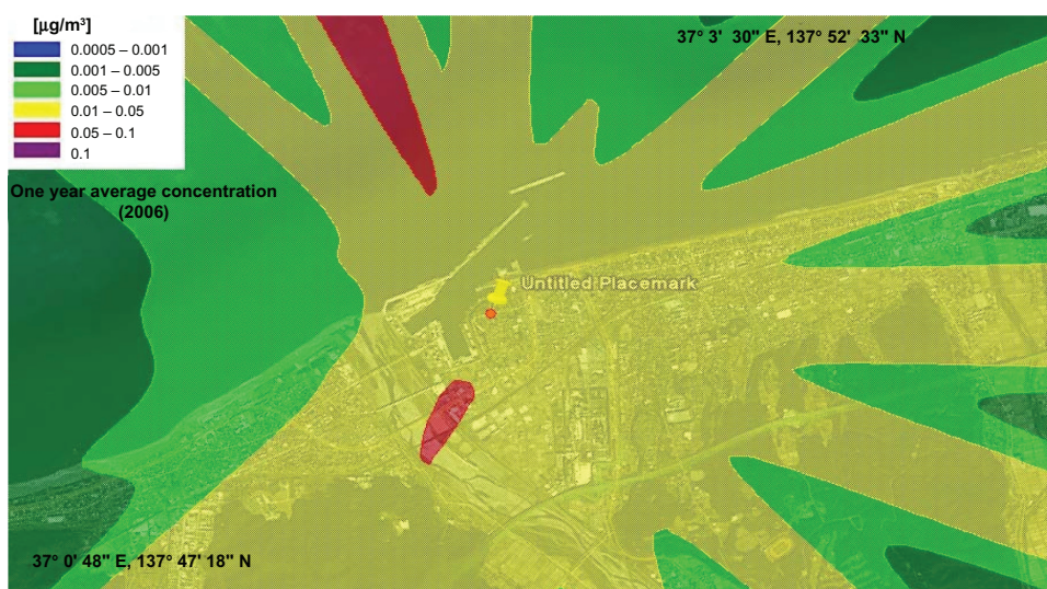
Figure 5. One-year average concentration distribution of mercury vicinity of a large point source in the coastal area of the Sea of Japan, calculated with the Ministry of Economy, Trade and Industry Low Rise Industrial Source Dispersion Model (METI-LIS) in 2006. The united place mark represents industrial source locations.
