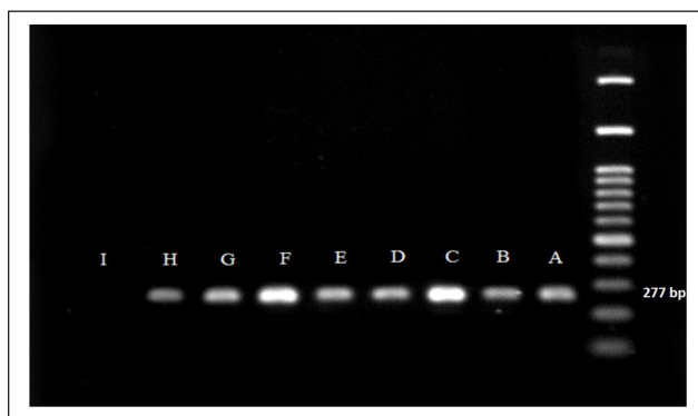
Figure 1 Agarose gel electrophoresis stained by ethidium bromide producing 277 base pair fragments for PKD1 mutant genes (A and B = positive control; C to H = PKD1 mutant genes; I = negative control)
