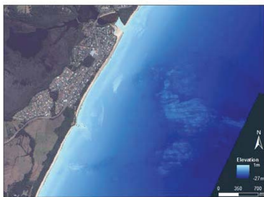
Figure 4. LiDAR data showing shoreface reef off Lake Cathie Beach.
