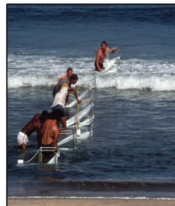
COVER PHOTOGRAPH: A field experiment coordinated by Nick Kraus in 1985 at Duck, NC called Duck’85. The researchers are busy with Nick’s ‘Streamer Traps’ that measure sand transported along the coast. As usual Nick is at the outer end of the measurement line near the most energetic breaking waves.
