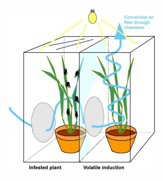
**Figure 1.** Chimney set-up to induce resistance by plant volatiles produced by plants infested with aphids. Left compartment completely closed but with a convention airflow trough with two (grey circular) screened parts. Right compartment with open top: the 'chimney' part.
