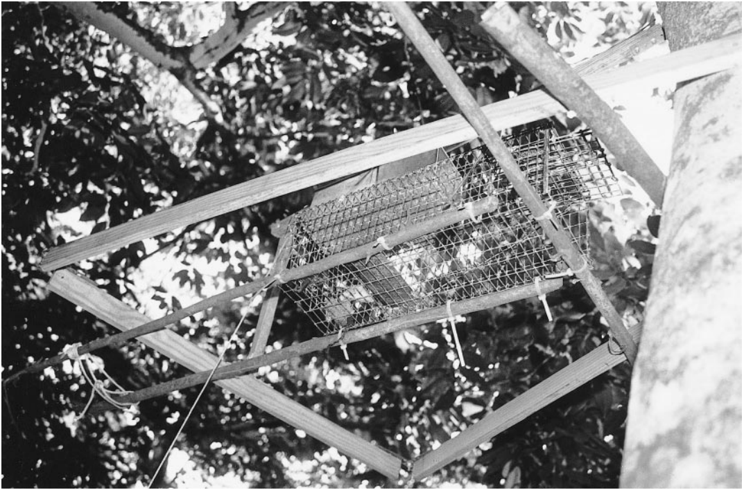
Fig. 5. Arboreal platform trap assembly in place at Paracou. Modified from Malcolm's (1991) basic design, each trap assembly consisted of one folding wire Tomahawk trap and a piggy-backed folding aluminum Sherman trap. Both are visible in this photograph, which resembles the perspective of an observer on the ground checking the traps with binoculars. Six species of marsupials and rodents were taken with this equipment, at heights ranging from 7.2 to 16.7 m above the ground.
