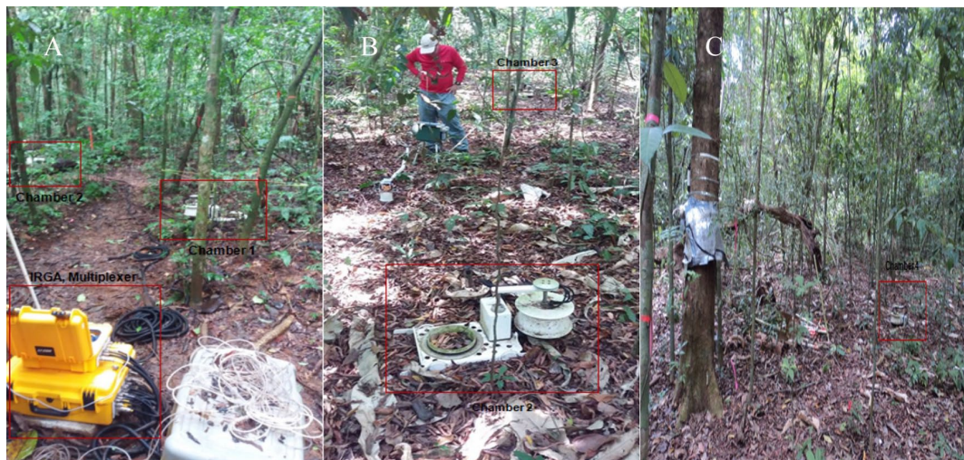
Figure 3. Photographs of the soil gas flux chambers used in this study: (A) infrared gas analyzer (IRGA) multiplexer device with chambers 1 and 2, (B) chambers 2 and 3, and (C) chamber 4.
