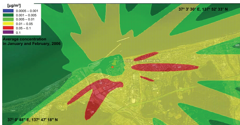
Figure 3. Average concentration distribution of mercury vicinity of a large point source in the coastal area in Japan Sea, calculated with the Ministry of Economy, Trade and Industry Low Rise Industrial Source Dispersion Model (METI-LIS) in January and February, 2006. The united place mark represents industrial source locations.
