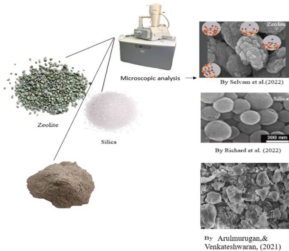
Figure 4. Micrography of zeolite, silica, and clay. Images from “Selvam et al., 2020, and Arulmurugan and Venkateshwaran, 2021” (used according to the Creative Commons Attribution 3.0 Unported License and STM permission guidelines, respectively), and “Richard et al., 2022” (used with permission from the Copyright Clearance Center’s RightsLink® service; Order Number: 5881860570738, Order Date: Oct 4, 2024).
