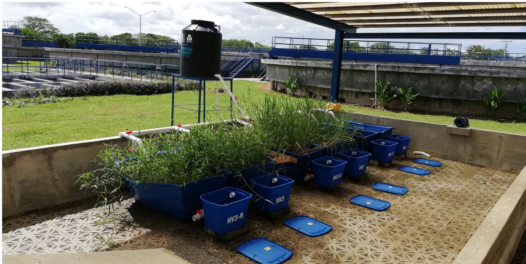
Figure 2. Artificial wetlands with horizontal subsurface flow using German grass (HV2/HV2-R) and Tanner grass (HV3/HV3-R).
