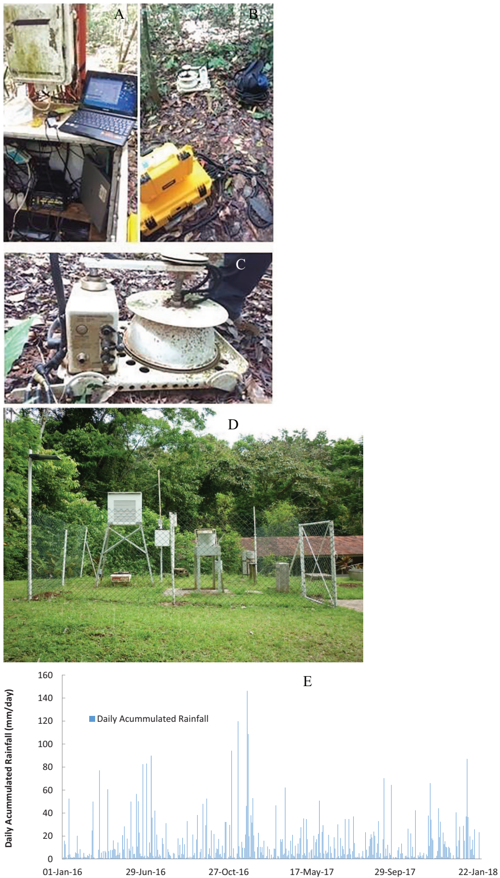
Figure 2. Research site in a 1 ha plot: (A) main eddy tower, (B) equipment used in this study, (C) soil gas flux chamber, (D) meteorological station called at El Claro, and (E) daily accumulated rainfall (mm) from January 2016 to January 2018. The rainy and dry seasons are evident from patterns in the data.
