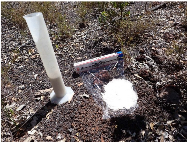
Fig. 3. The method for determining the volume of soil displaced by each echidna ( Tachyglossus aculeatus ) dig using a known volume of clean, washed river sand to fill the dig and determine the actual volume of soil displaced. Photo was taken at one of the study sites in the Northern Jarrah Forest, south-western Australia (photo credit: S. Dundas).
